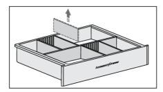
Wooden dividers in the drawer can be inserted into the grooves to fit the accessories you are storing (bottle opener, pourer/spout, wine stoppers etc.).
