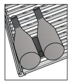
In some cases, during opening/closing of the shelf, bottles are not properly positioned or stopped and they can move. To prevent movement of the bottles on the shelf, it is recommended to use the accessory 'bottle stopper' (a) included in the appliance equipment.
