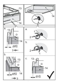
If the shelf (13) and drawer (14) are not aligned at the front ( $d\neq 0$ ), first completely pull out the drawer to access the drawer opening mechanism on the back wall. Press on the spacer (A) to release the mechanism. Rotate the spacer to adjust the length.
