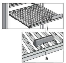
The wooden bottle shelf with moon shaped recesses allows you to load the bottles onto the shelf cross-wise.
