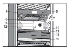
The serving area (zone B) is a temperature zone between the top (5) and bottom (15) insulation barrier. It allows you to bring the wine on ideal consumption temperature, and to prepare in advance everything you need for quick and top-notch wine serving: chilled wine glasses, space for already open bottles, decanter, and other accessories (bottle openers, wine pourers/spouts, stoppers ...).
