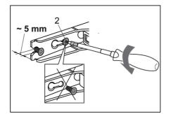
3. Partly (by no more than 5 mm) undo the hinge screws (2) at the top and bottom. Do not completely undo the screws. This way, the door will remain in contact with the housing.
