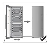
15. Close the door and make sure it is aligned with the housing. The housing side and the edge of the door should be parallel.
