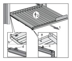
To remove a shelf from the appliance, fully extend the telescopic rails (1), and then vertically lift the shelf (2) to remove it from the rails. Take care not to damage the door gasket.
