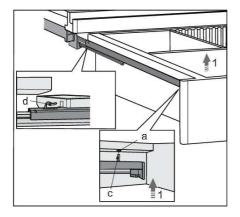
The drawer can also be removed from the appliance without removing the serving bottle shelf from its rails. To do this, fully open the drawer, lift it at the front (1) and pull it towards you.
