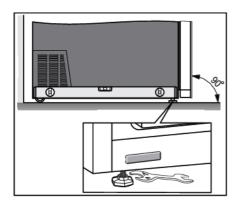
When the appliance is placed on the intended surface, it should be completely level in order to decrease vibration. To level the appliance, use the adjustable feet at the front of the appliance. An open wrench size 17 is required for adjusting and fastening the feet.
