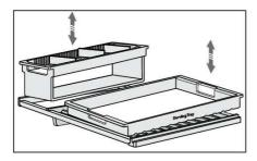
Inclination serving bottle shelf (13) is installed on the full-extension telescopic rails with soft close and it is secured against tipping over. A serving tray is placed on the front part of the serving shelf, and the vertical bottle holder is inserted into the shelf's rear part. The tray and the bottle holder can be lifted and removed from the support shelf (for serving purposes outside the Wine Climate Cabinet, maintenance or cleaning).
