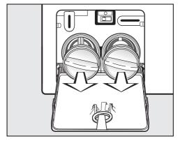
■ Remove the drain filters completely.
