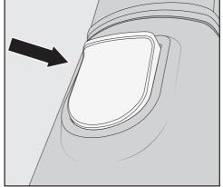
■ To separate the individual sections from each other, press the release catch on the Electrobrush and pull the connector out of the Electrobrush.
